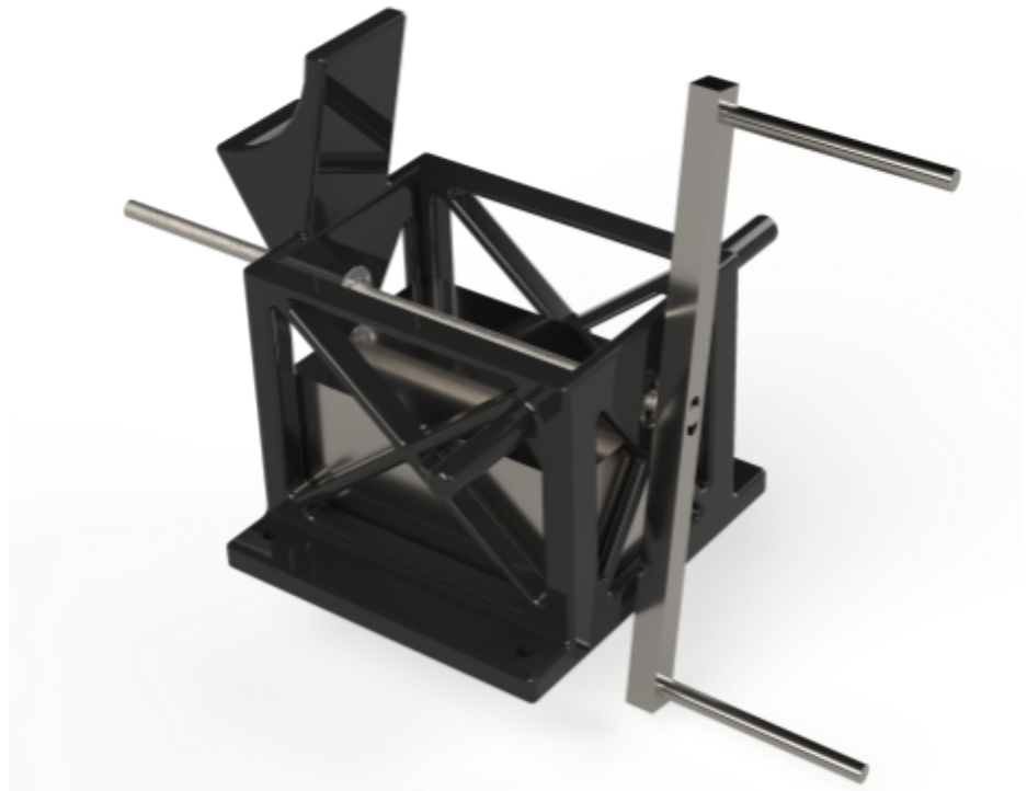
Figure [13]: Rear support, counter weights, and handle.
