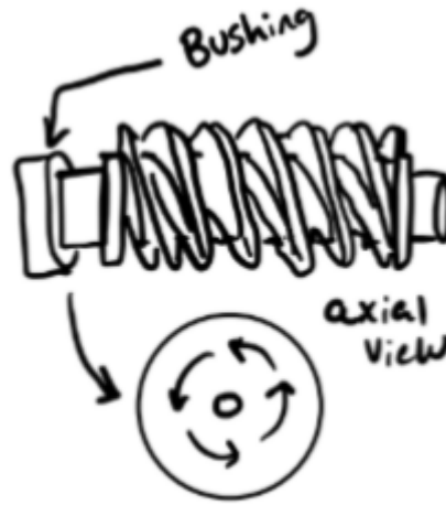
Figure [16]: Friction between worm gear and HDPE bushing.
