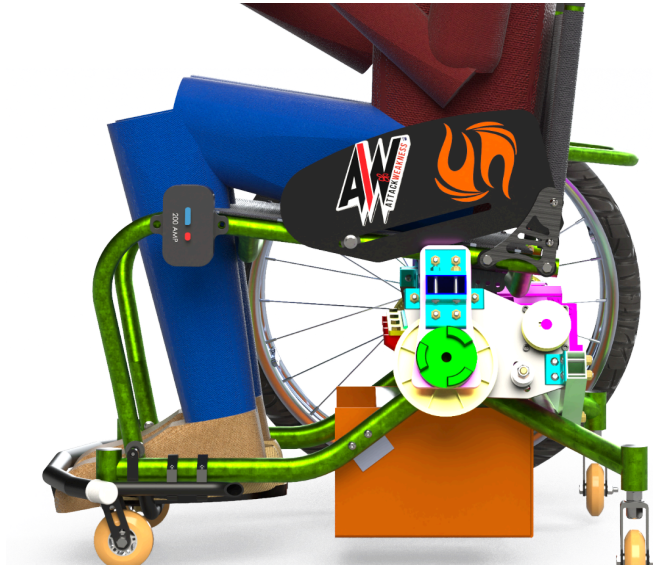
Figure 12: Side View of Wheelchair Showing Battery Mount Location
