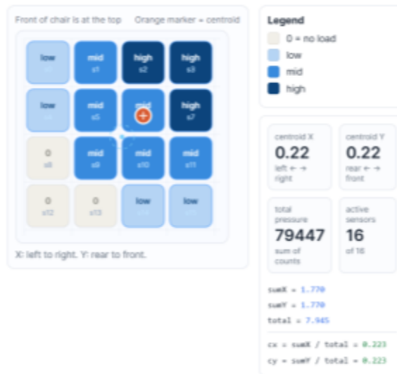
Figure 8: Example pressure detection using a 4x4 array.
